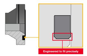
The EFS fits precisely in Code 61 and Code 62 flanges because its shape and size are engineered for the space and application. Its purpose-designed shape reduces the possibility of pop out, and the need to replace or reinstall the O-ring, eliminating costly leakage and time consuming pre-assembly handling.
