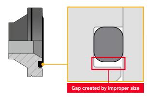
Standard O-rings have an unnatural fit in Code 61 and Code 62 flanges because of their improper size and shape. This off-the-shelf solution creates a gap which can lead to difficult installation, hose assembly leakage and the potential for the O-ring to fall out.
